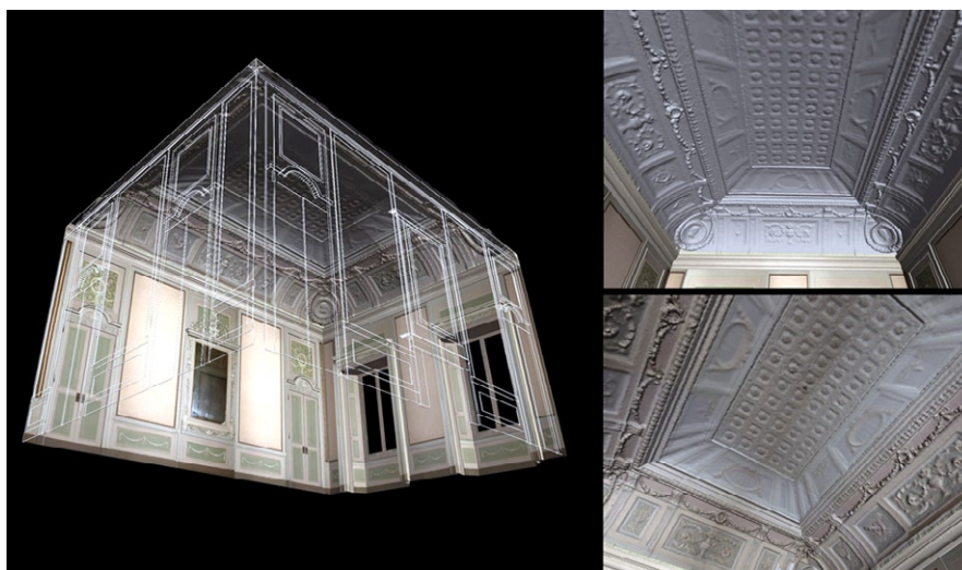
Fig. 6. Virtual model of a room with photogrammetric images used as textures.
