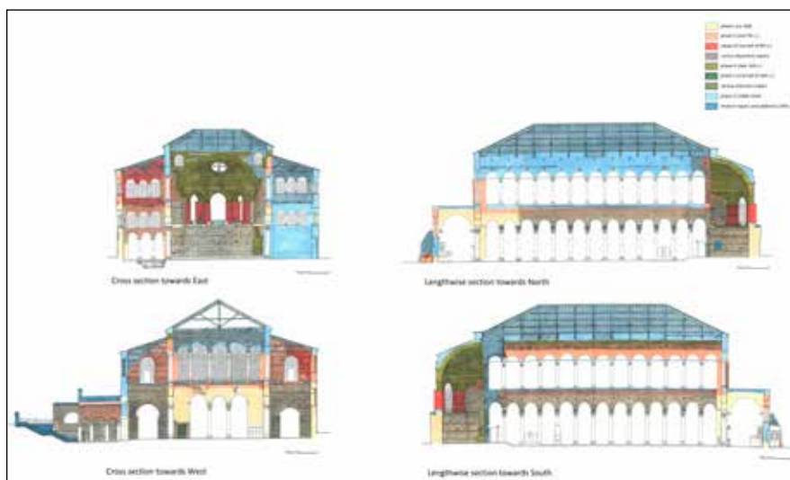
Fig. 6 Acheiropoietos basilica. Structural phases: sections.
